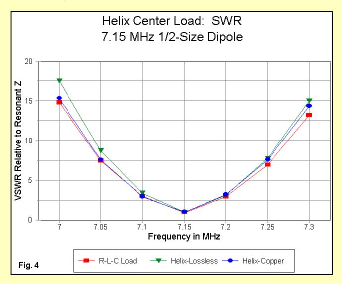
Despite the lower Q estimate, the source impedance of the physically modeled helical loaded dipole is lower than even the Type 0 model at zero load loss. As **Fig. 4** shows, the SWR curve is slightly steeper than even the R-L-C lossless load model--and a lossless helix yields a steeper curve yet.
