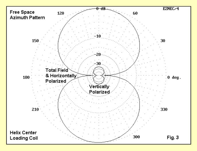
The small but definite vertically polarized radiation field results from radiation from the portions of the helix that are vertically oriented. This field alone would not suffice to provide the added gain
