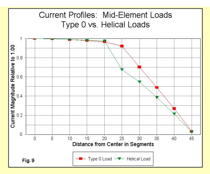
Despite the close correspondence of current up to the load position and the dramatically lower current beyond that point for the physically modeled helix, the model shows a significantly higher gain than either the corresponding Type 0 load model or even the physically modeled center load. The following table summarizes the gain situation for various models.
